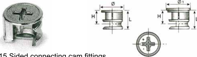
Ø15 Sided connecting cam fittings Finish:Zn-plated, NI-Plated Mat:Zn-Alloy
